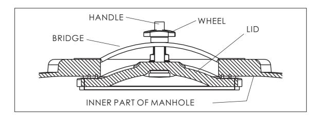
Introduce the lid in the manhole, leaving it leveled and centered. The lid must be supported by the handle, as this will avoid that it could fall into the tank and damage any of its parts.
