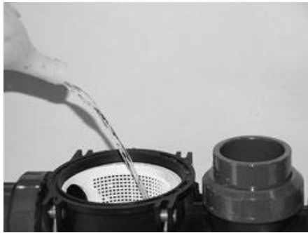
Prime the pump (if not risk of dry running). GUARANTEE LOSS.
