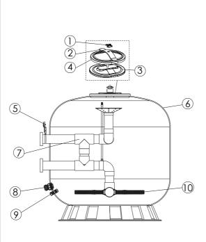
Notes: 10\* 06831200 should have 185mm x 8pcs and 233mm x 8pcs and 129mm x 8pcs of laterals 10° 06831400 should have 185mm x 4pcs and 233mm x 12pcs and 129mm x 12pcs of laterals 10° 06831600 should have 185mm x 8pcs and 233mm x 12pcs and 129mm x 12pcs of laterals
