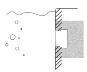
1. Put the sleeve into the wall, the topper side need on same level with wall surface, cable need to go through the sleeve and request 30cm gravel drainage layer
