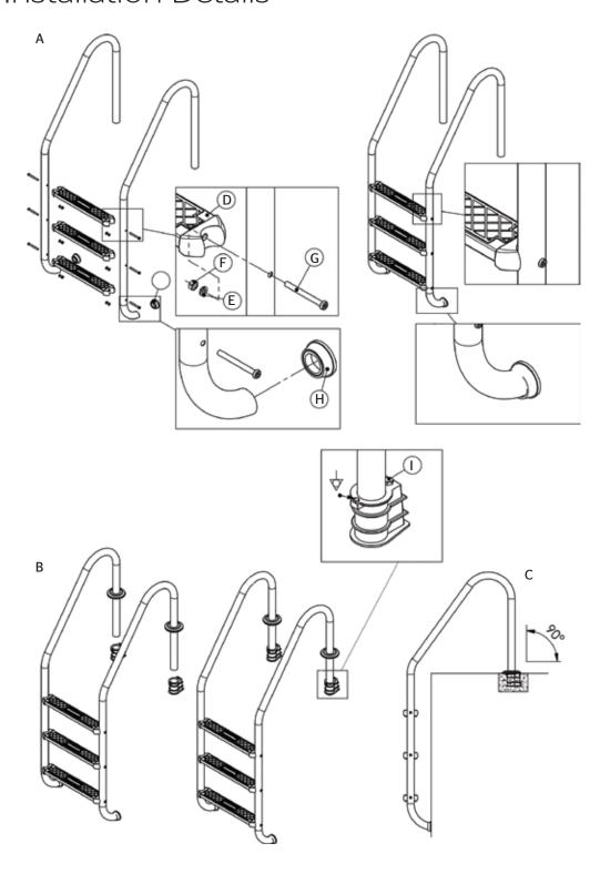
1.Assemble the ladder, positioning the threads(d) and fixing same by means of the corresponding screws(g), nuts (f) and washers(e).
