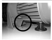
Check regularly the watertightness! (An escape for the shaft seal causes important damages).
