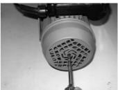
In order to avoid blockades of the shaft seal, please rotate the axis through the impeller before the beginning or after prolongated stoppings.
