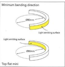
LED Neon flex is a highly durable product but must be installed in accordance to the pictures shown below, which indicate the minimum bending parameters as well as the correctly bending direction for each specific variant of model
